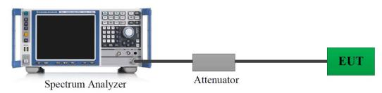
A short RF cable with low cable loss connected to the EUT antenna port, which was provided by manufacturer.
