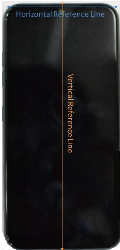
SAR Test Setup Photo 17: Horizontal and Vertical Reference Lines
