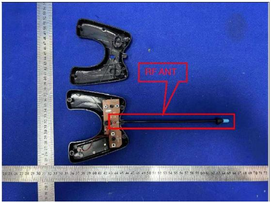
Length: 21cm Antenna Type: Spring Antenna Antenna Gain: 0dBi
