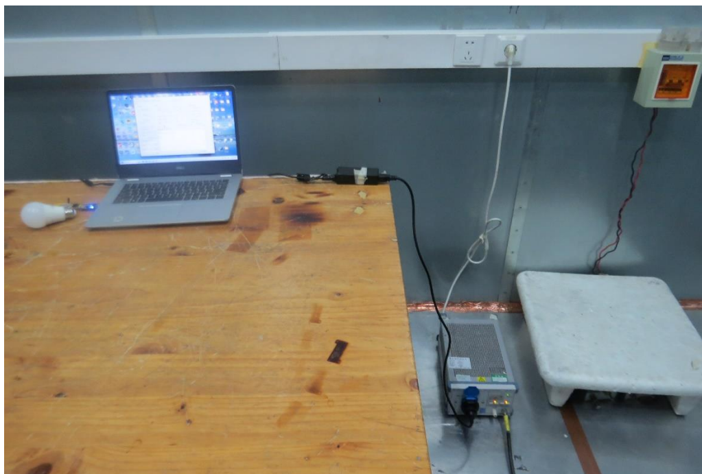
Picture 2 Conducted Emission Test Setup
