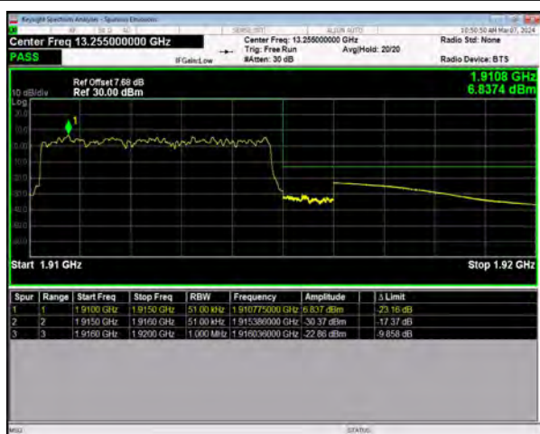
n25 SCS=15kHz DFT_16QAM BW=5MHz HighChannel=382500 RB=25@0
