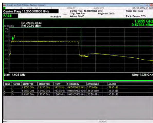
n25 SCS=15kHz CP_QPSK BW=10MHz HighChannel=382000 RB=52@0
