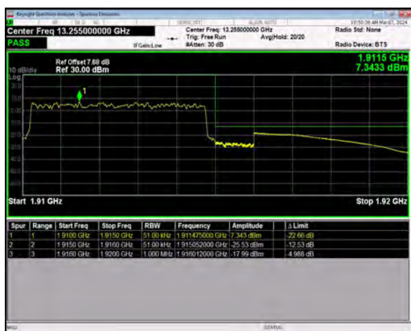
n25 SCS=15kHz DFT_QPSK BW=5MHz HighChannel=382500 RB=25@0
