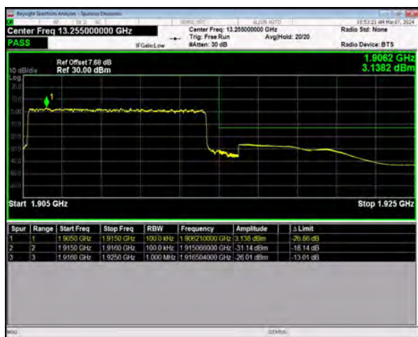
n25 SCS=15kHz DFT_BPSK BW=10MHz HighChannel=382000
