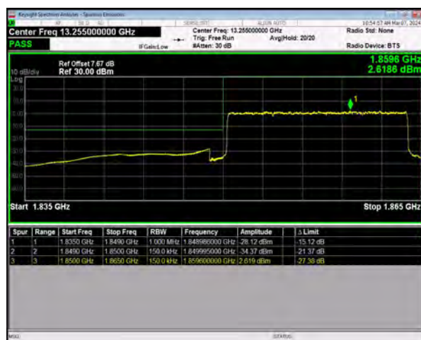
n25 SCS=15kHz DFT_BPSK BW=15MHz LowChannel=371500 RB=75@0
