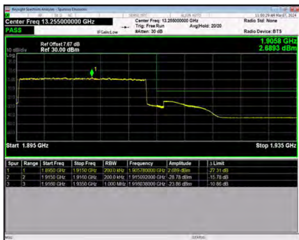
n25 SCS=15kHz DFT_QPSK BW=20MHz HighChannel=381000 RB=100@0
