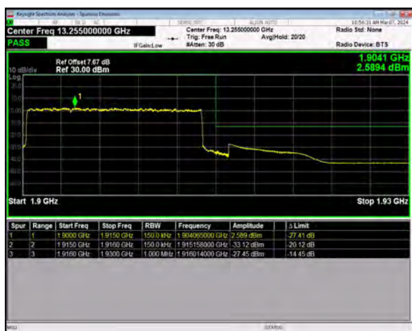
n25 SCS=15kHz DFT_BPSK BW=15MHz HighChannel=381500 RB=75@0
