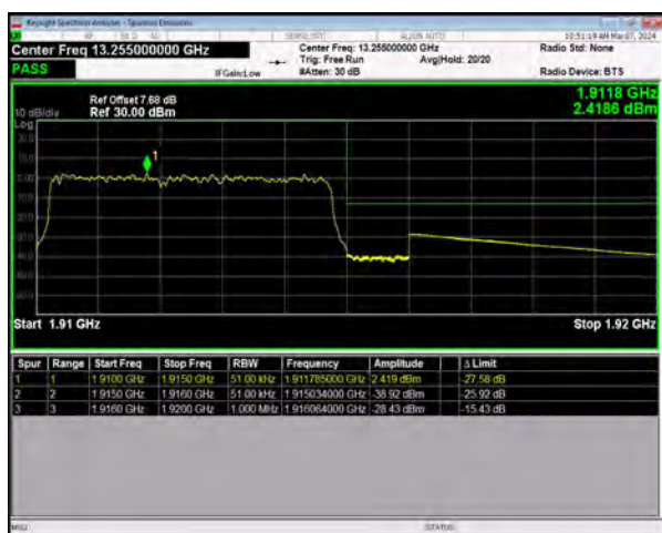
n25 SCS=15kHz DFT_256QAM BW=5MHz HighChannel=382500 RB=25@0
