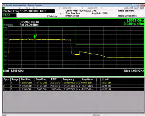
n25 SCS=15kHz DFT_16QAM BW=20MHz HighChannel=381000 RB=100@0
