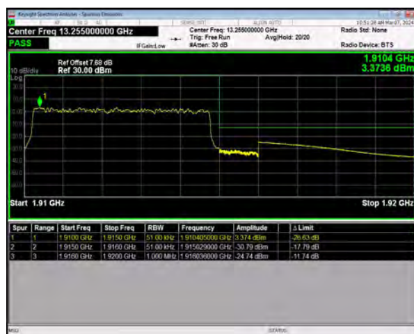
n25 SCS=15kHz CP_QPSK BW=5MHz HighChannel=382500 RB=25@0
