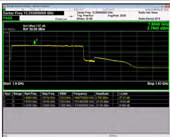
n25 SCS=15kHz DFT_QPSK BW=15MHz HighChannel=381500 RB=75@0
