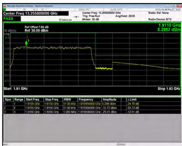
n25 SCS=15kHz DFT_64QAM BW=5MHz HighChannel=382500 RB=25@0
