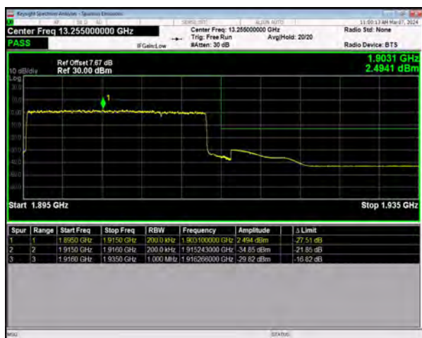
n25 SCS=15kHz DFT_BPSK BW=20MHz HighChannel=381000 RB=100@0
