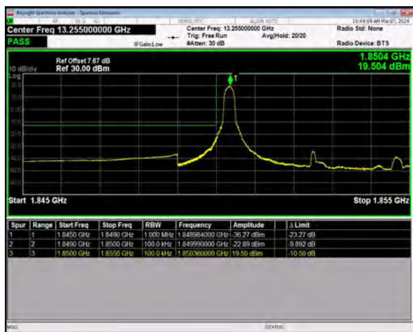
n25 SCS=15kHz DFT_QPSK BW=5MHz LowChannel=370500 RB=1@0
