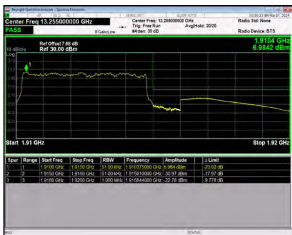
n25 SCS=15kHz DFT_BPSK BW=5MHz HighChannel=382500 RB=25@0
