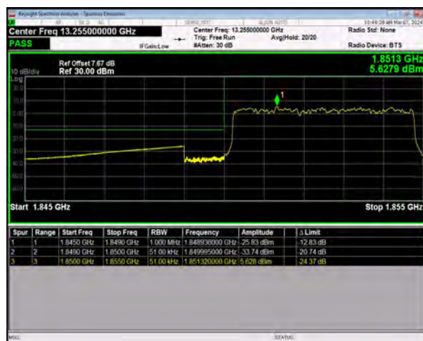
n25 SCS=15kHz DFT_16QAM BW=5MHz LowChannel=370500 RB=25@0
