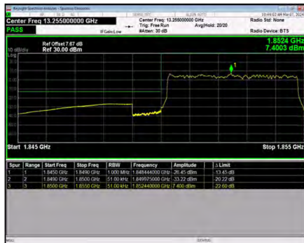
n25 SCS=15kHz DFT_BPSK BW=5MHz LowChannel=370500 RB=25@0
