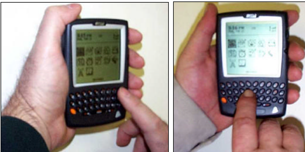
Figure 3. Users of the Proton pager holding the pager in their left hand and typing with their right forefinger.
