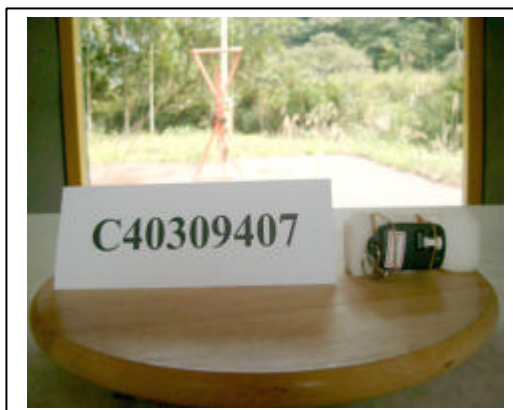
Radiated Open Site Test Set-up
