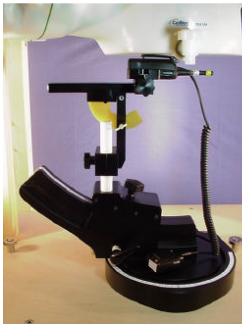
Body SAR Test Setup with SAM Planar Phantom
