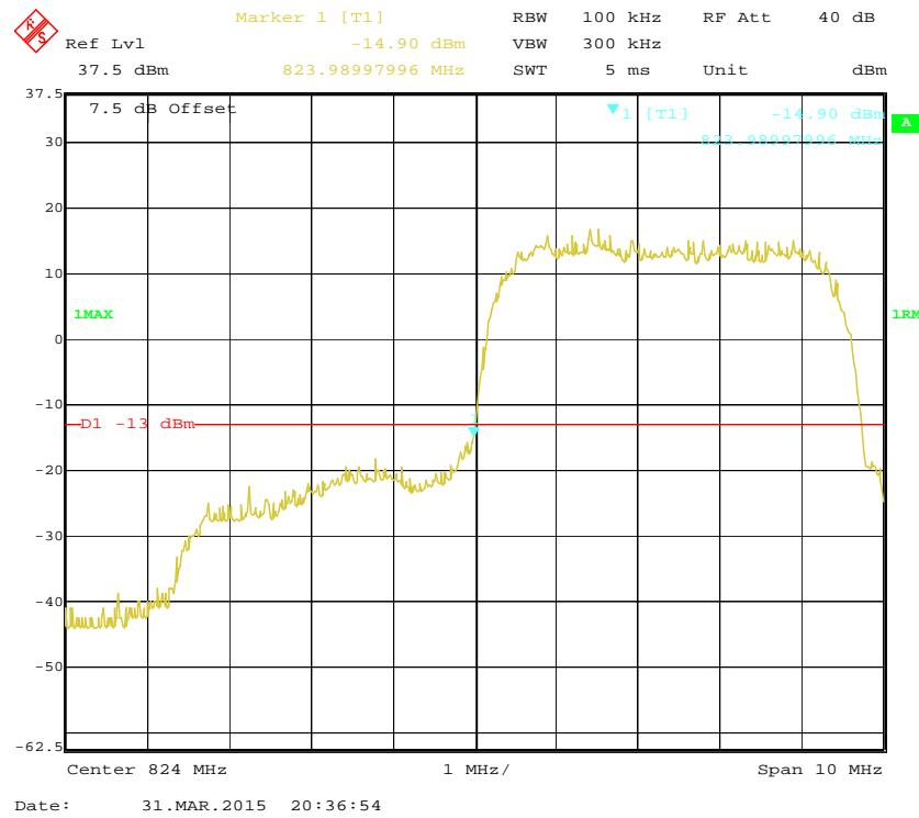
**Cellular Band, Right Band Edge for WCDMA (QPSK) Mode**
