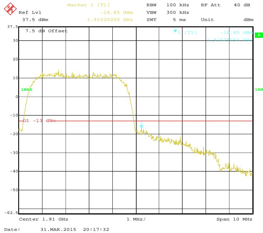
**PCS Band, Left Band Edge for HSUPA (QPSK) Mode**
