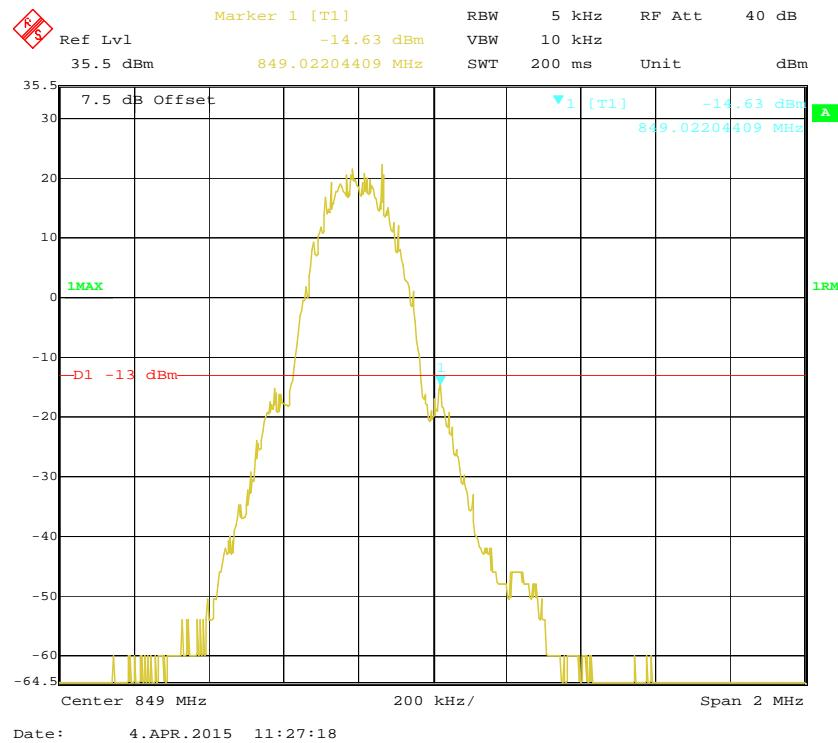
**Cellular Band, Left Band Edge for EGPRS (8PSK) Mode**
