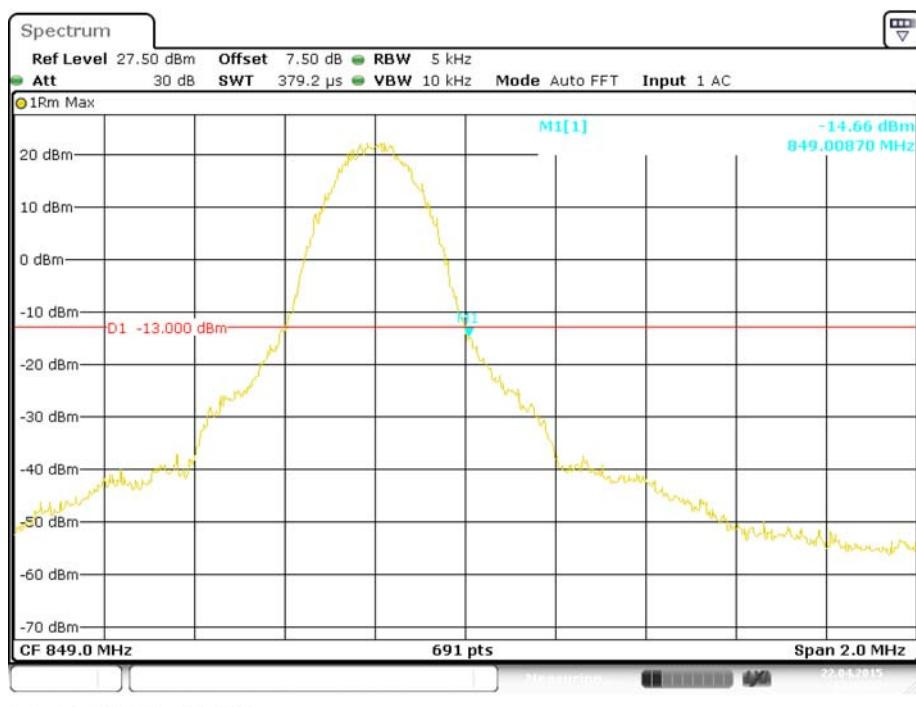
**Cellular Band, Left Band Edge for WCDMA (QPSK) Mode**
