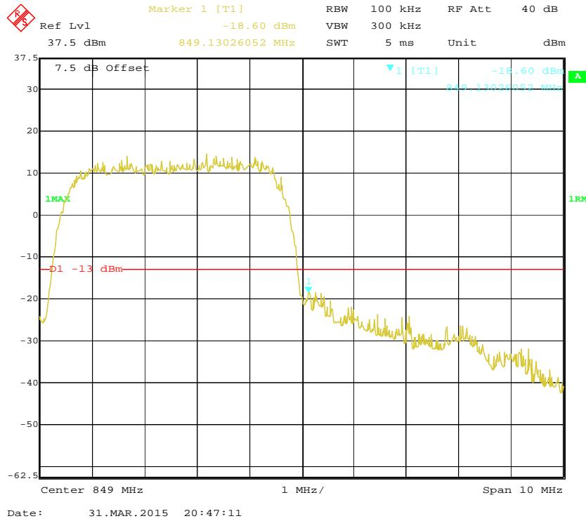
**Cellular Band, Left Band Edge for HSUPA (QPSK) Mode**
