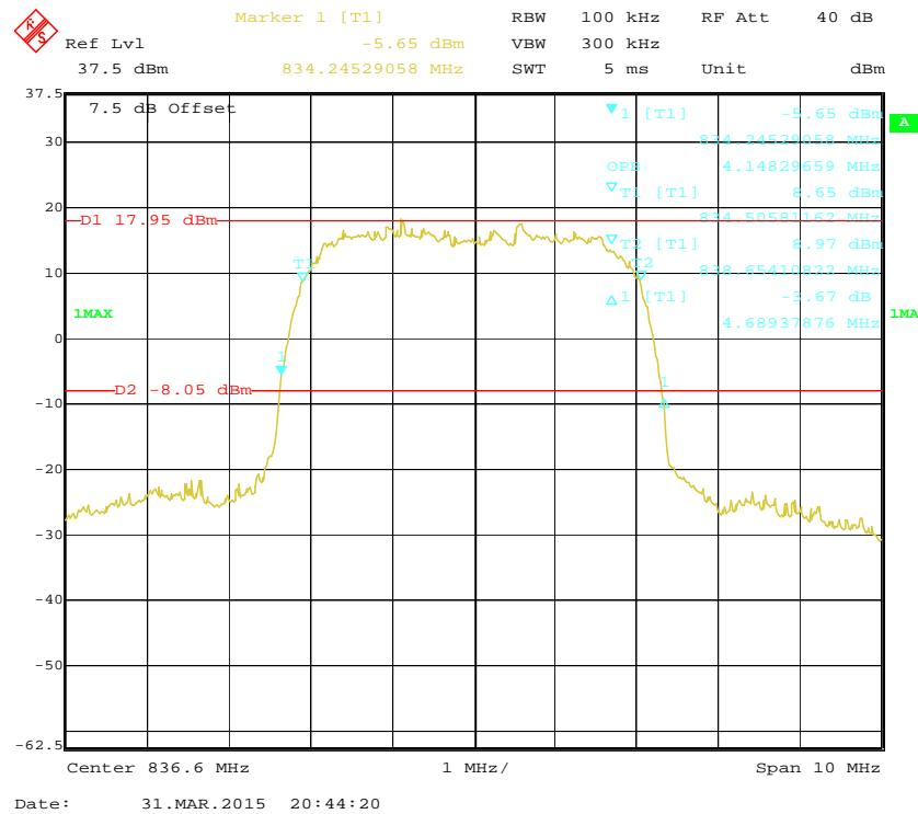
**99% Occupied & 26 dB Emissions Bandwidth for HSDPA (16QAM) Mode**
