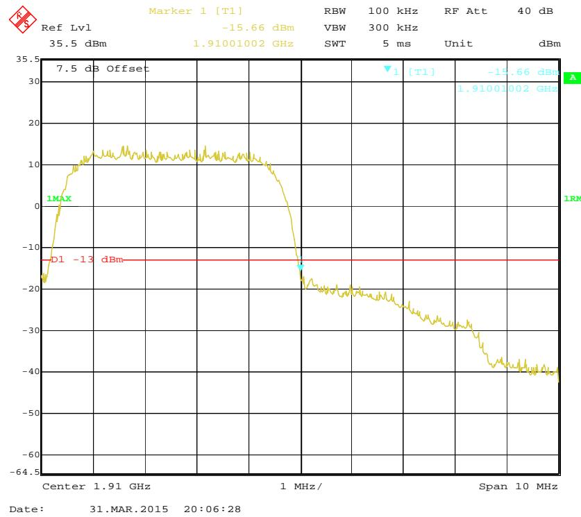
**PCS Band, Left Band Edge for HSDPA (16QAM) Mode**
