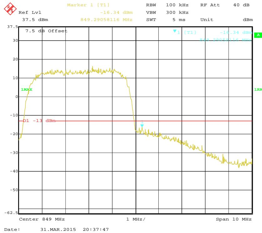
**Cellular Band, Left Band Edge for HSDPA (16QAM) Mode**
