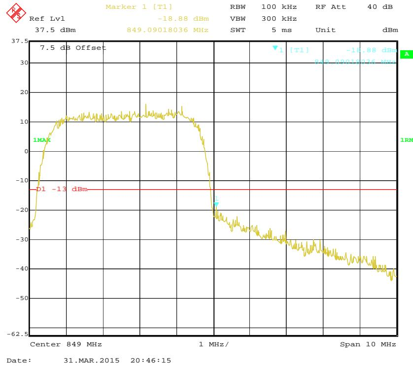
**PCS Band, Left Band Edge for GSM (GMSK) Mode**
