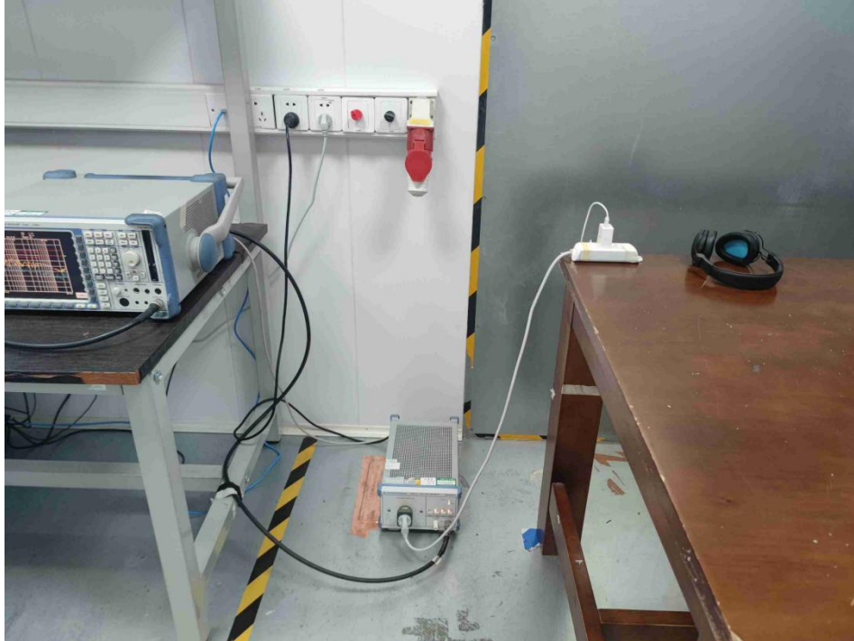
Conducted emissions at AC power line (150kHz-30MHz)
