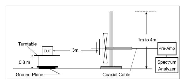
Radiated Emission Test Set-Up, Frequency Above 1GHz.
