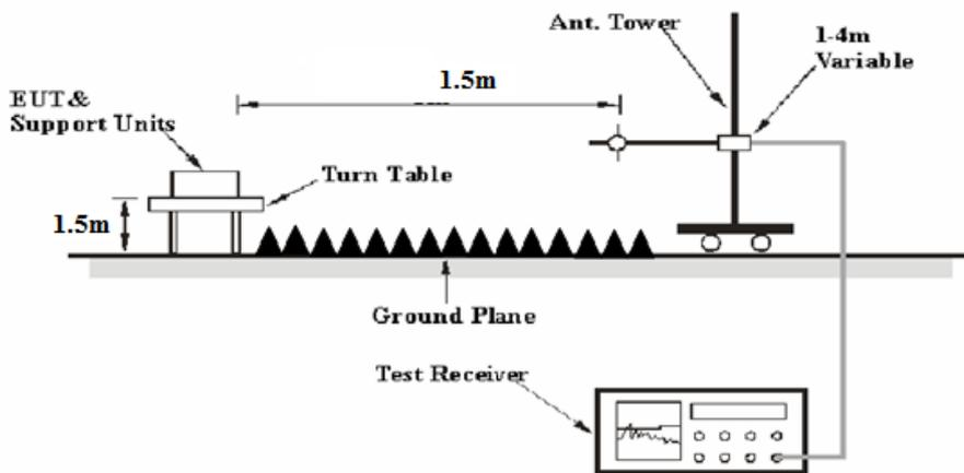
The radiated emission Below 1GHz tests were performed in the 10 meters chamber test site, above 1GHz tests were performed in the 3 meters chamber test site, using the setup accordance with the ANSI C63.10-2013. The specification used was the FCC 15.209, and FCC 15.407 limits.
