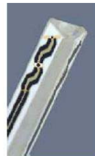
Figure 3.3 Probe Thick-Film Technique
