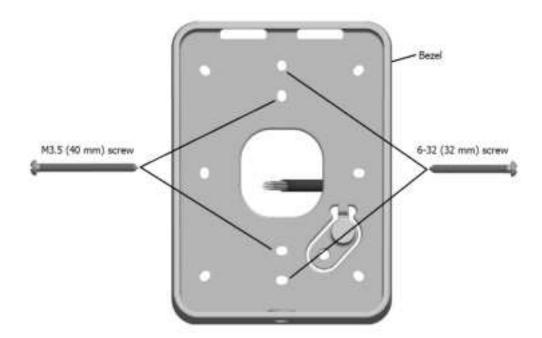
4. Drill pilot holes for the four corner fixing holes and the tamper tab. Secure the bezel to the mounting surface using the four corner fixing screws provided. Secure the tamper tab (located in the bezel) to the mounting surface using the remaining fixing screw provided. It is important the four corner fixing screws are used to ensure the reader is flush with and tight against the mounting surface.
