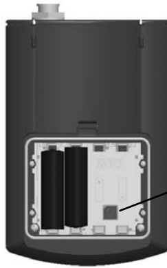
Figure 6. Rotary Switch in Battery Cradle
