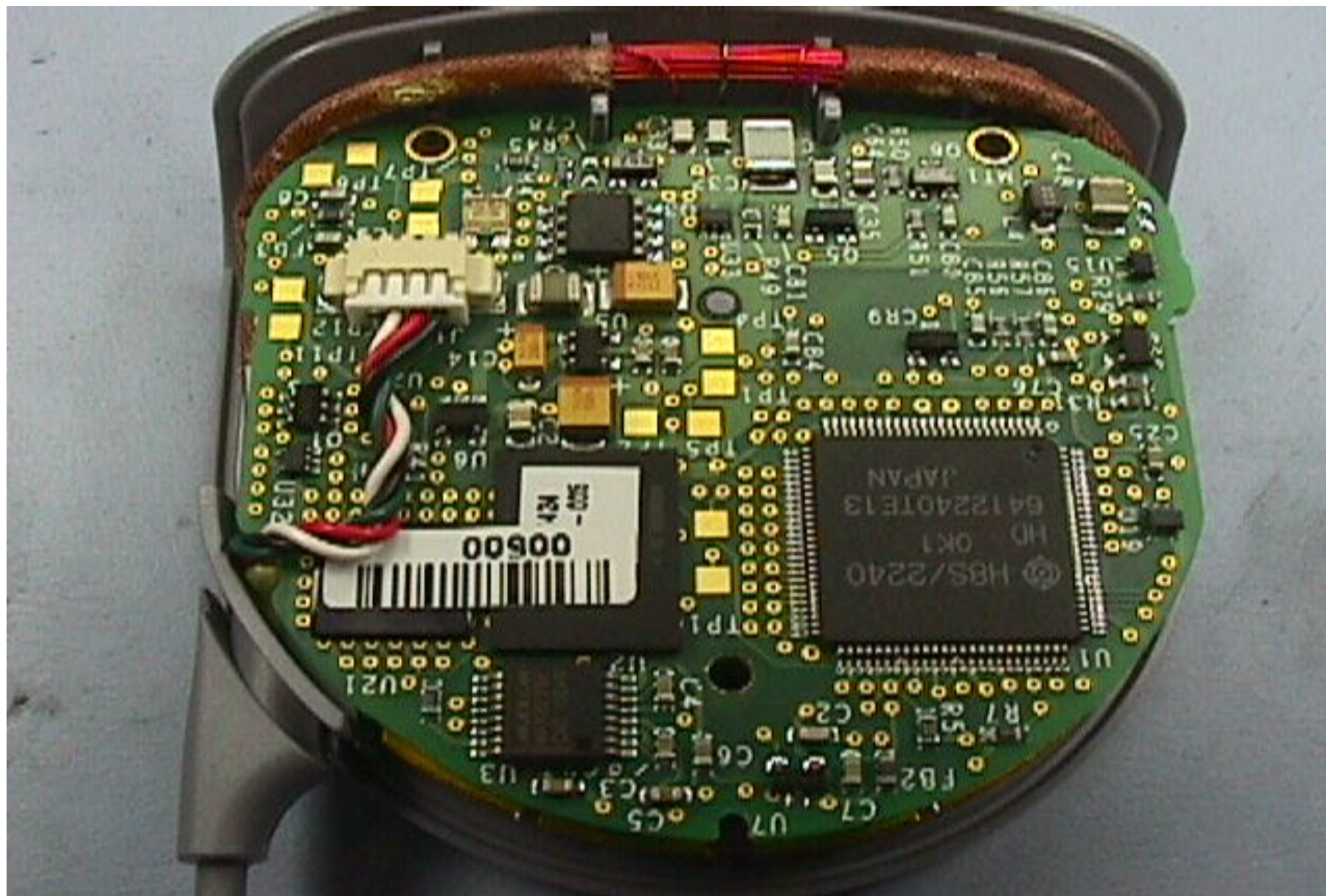
2490A Telemetry Module Circuit Board, Top Side
