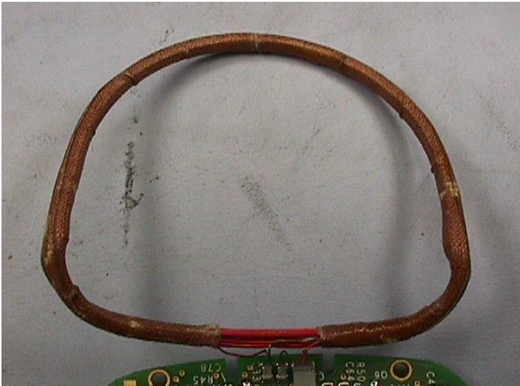
2490A Telemetry Module Antenna Coil
