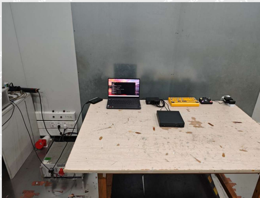
Conducted emissions on AC mains
