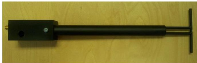
Figure 1 – MVG COMOSAR Validation Dipole
