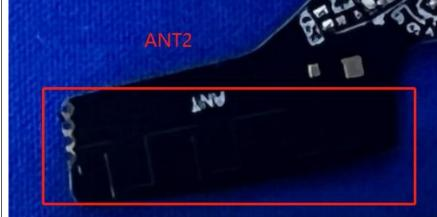
The antenna is PCB antenna.
