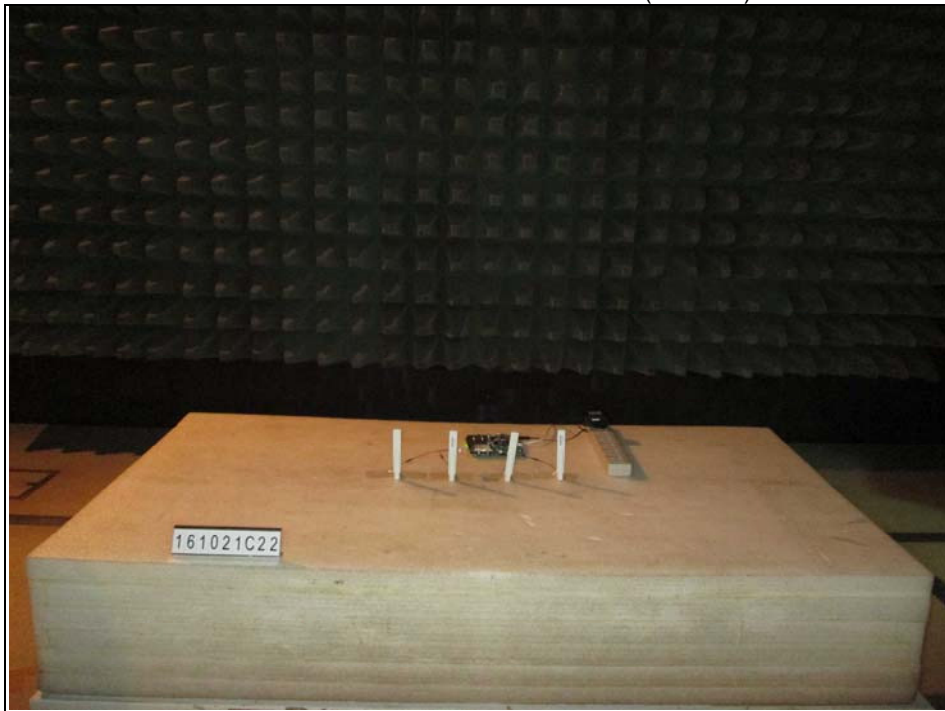
Radiated Emission Test below 1GHz (Mode B)
