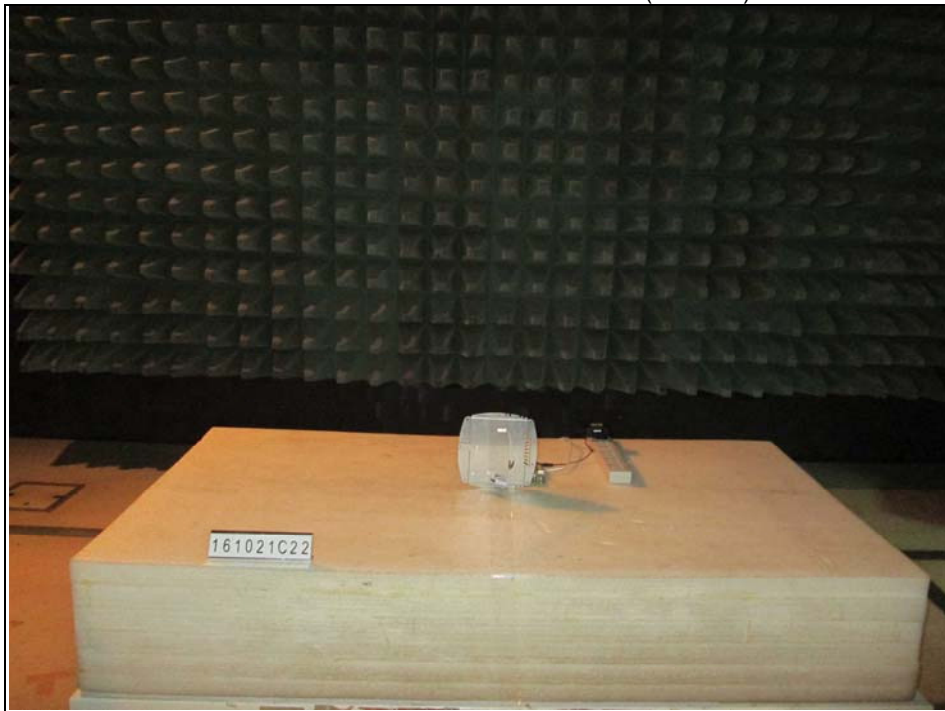
Radiated Emission Test below 1GHz (Mode A)
