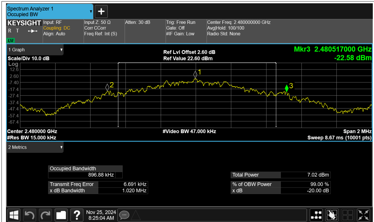
-20dB Bandwidth NVNT 2-DH1 2402MHz Ant1
