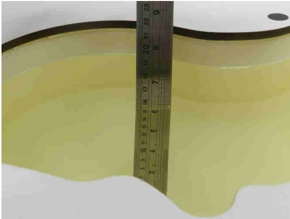
Fig 11.1 Photo of Liquid Height for Head SAR
