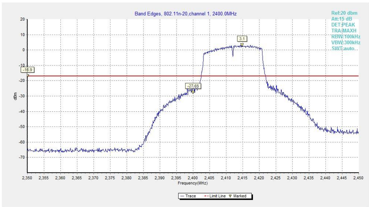
Fig.A.5.5 Band Edges (802.11n-HT20, Ch 1)
