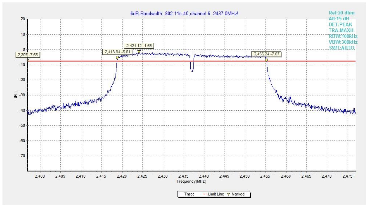
Fig.A.4.11 Occupied 6dB Bandwidth (802.11n-HT40, Ch 6)
