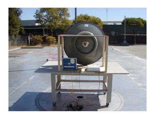
Radiated Emission – with antenna MA-WA58-1X
