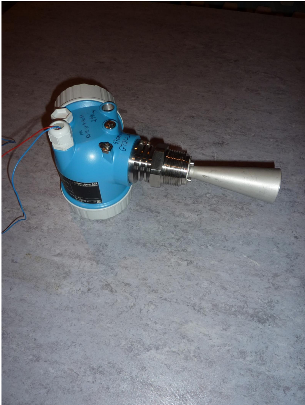
172289_106.JPG: ProToF BTLE-adaptor 2.4 GHz inside FMR51, test setup fully anechoic chamber (pos. 2, 40 GHz to 100 GHz)
