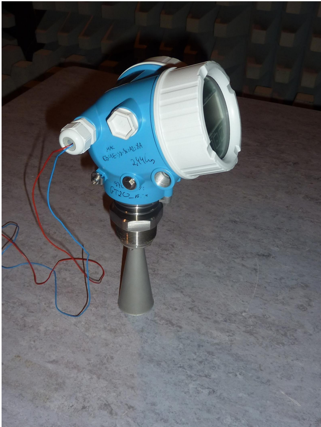
172289_105.JPG: ProToF BTLE-adaptor 2.4 GHz inside FMR51, test setup fully anechoic chamber (pos. 1, 40 GHz to 100 GHz)
