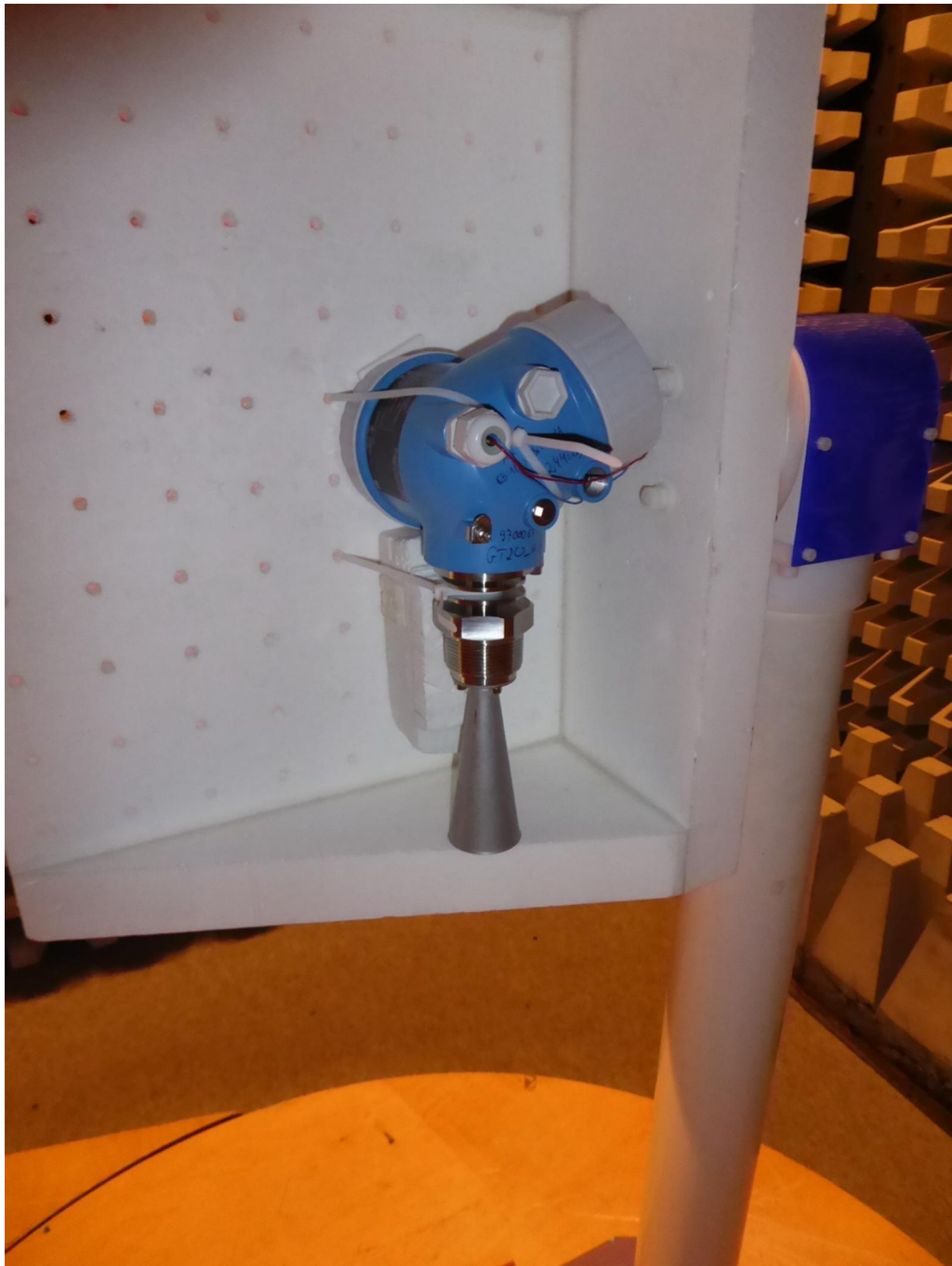
172289_100.JPG: ProToF BTLE-adaptor 2.4 GHz inside FMR51, test setup fully anechoic chamber (pos. 1)
