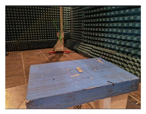
Radiated Emission above 1GHz test:
