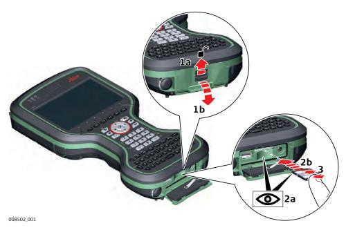
The SD card can be inserted into a slot behind the connector cover.
