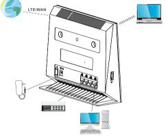
Step 1 Connect the power adapter to the CPE.
