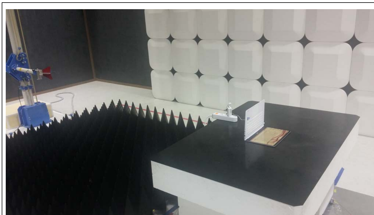
Material of Black plate: Plastic (Non-conductive material)
