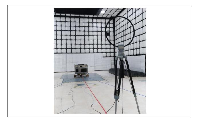
• Radiated Test Picture (Back): Below 30 MHz
