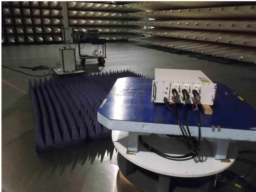
Test setup: Field Strength Emission 1 - 18 GHz @3m in the SAC
