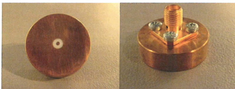
Figure 1 – MVG LIMESAR Dielectric Probe
