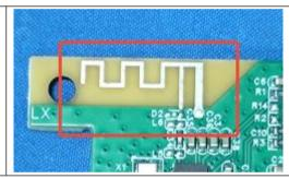
The antenna is PCB antenna.
