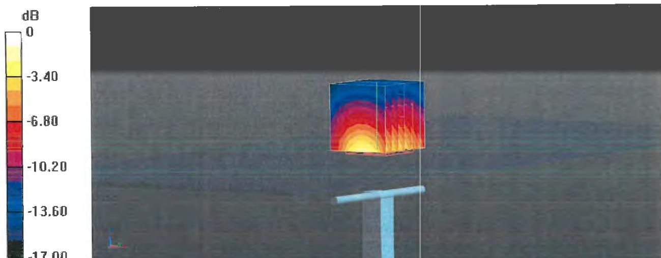
$$0 \text{ dB} = 14.5 \text{ W/kg} = 11.61 \text{ dBW/kg}$$
