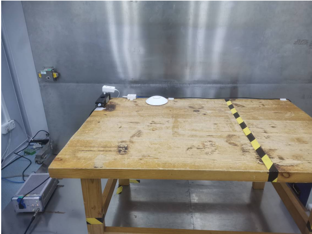
Conducted Emissions Side View- Powered by 802.3af POE
