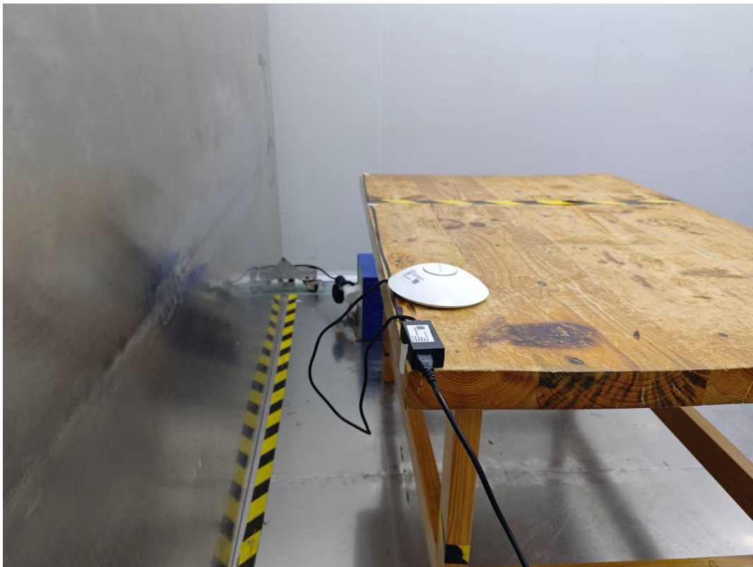
Conducted Emissions Side View-Powered by 24V POE
