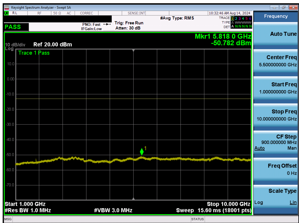
Plot 7-26. Conducted Spurious Plot (UMTS Ch. 4458)
