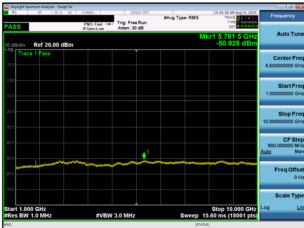
Plot 7-23. Conducted Spurious Plot (UMTS Ch. 4408)
