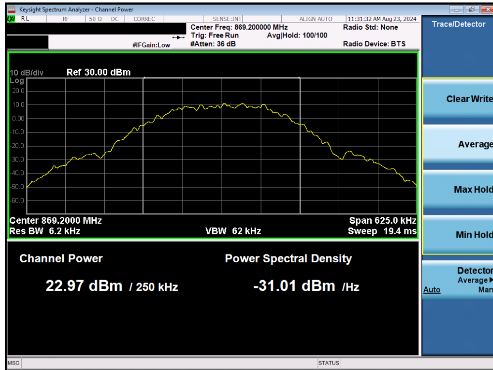
Plot 7-4. Conducted Power Output Data (GSM 850 – Low Channel)
