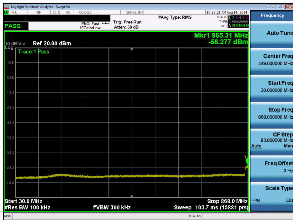
Plot 7-24. Conducted Spurious Plot (UMTS Ch. 4458)
