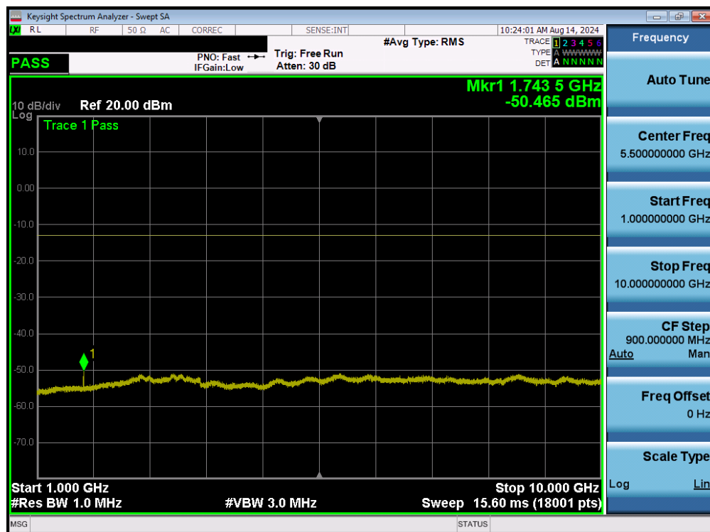
Plot 7-20. Conducted Spurious Plot (UMTS Ch. 4357)
