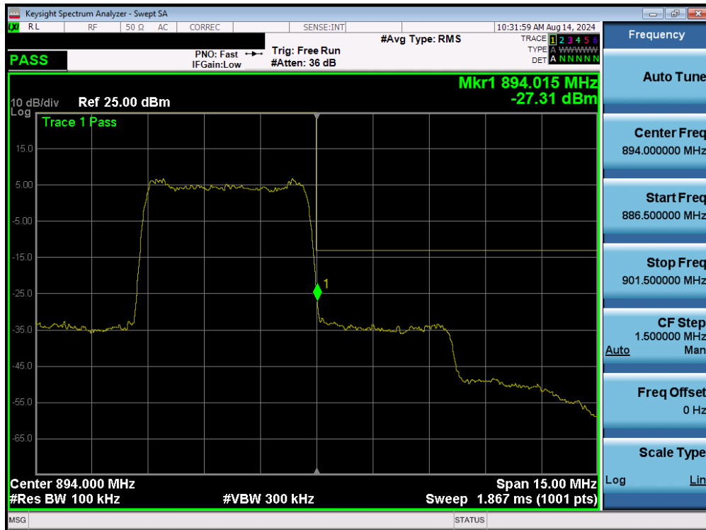
Plot 7-30. Upper Band Edge Plot (UMTS Cell – Ch. 4458)
