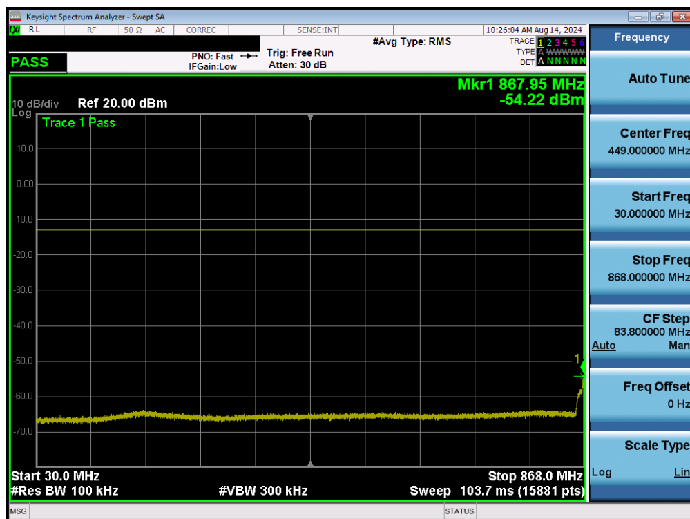
Plot 7-21. Conducted Spurious Plot (UMTS Ch. 4408)
