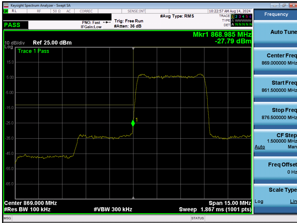
Plot 7-29. Lower Band Edge Plot (UMTS Cell – Ch. 4357)
