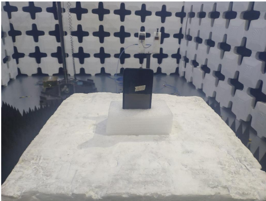
10. Radiated Emissions (Part 15C, 18GHz -26.5GHz)
