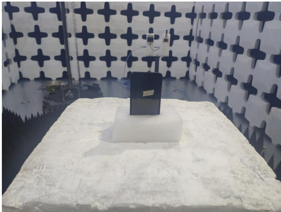
12. Radiated Emissions (Part 22/24/27, 18GHz -26.5GHz)
