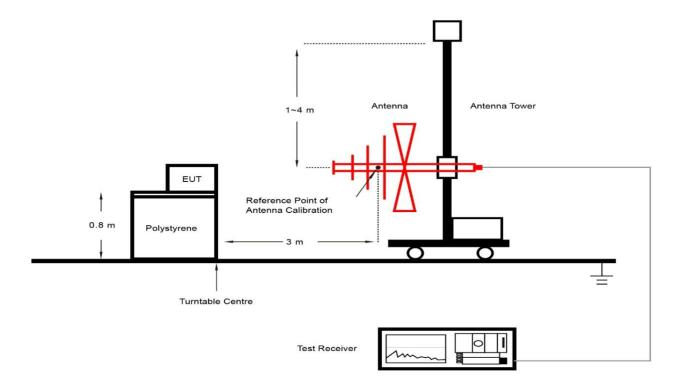
Above 1GHz Test Setup:
