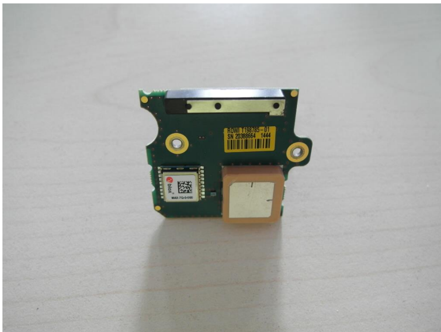
Photo 10: Antenna module with GPS chip
