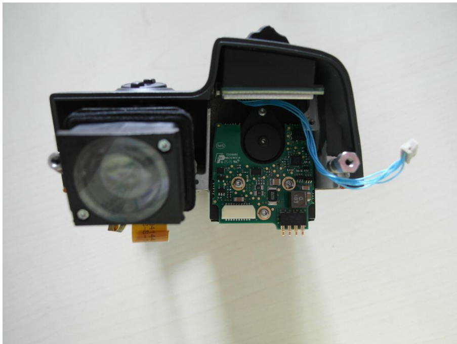
Photo 19: View finder and the battery connector board
