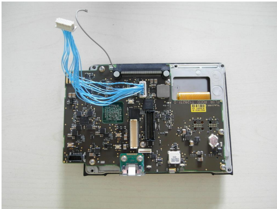
Photo 23: computer board with cable to battery connector board
