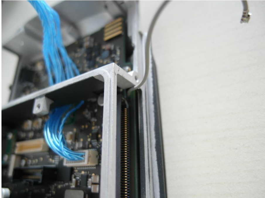
Photo 21: UFL RF cable thru the housing
