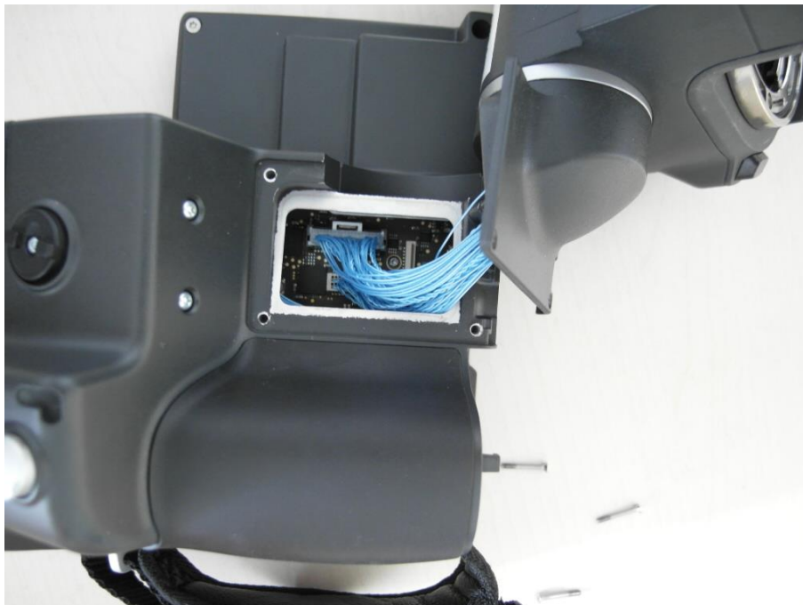
Photo 1: separation of main body and radiometric unit
