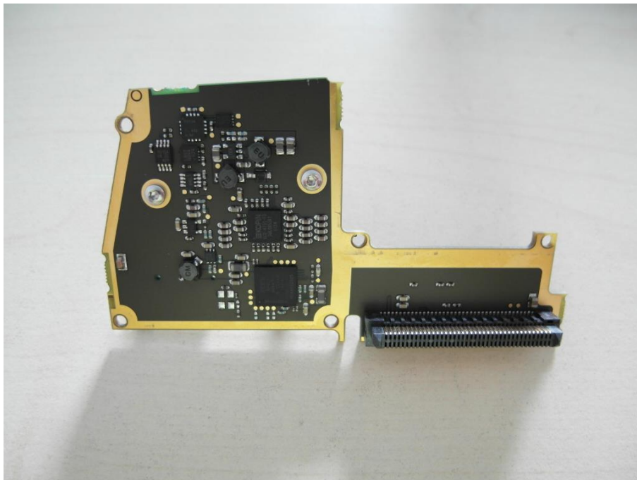
Photo 17: connector board between view finder and computer board
