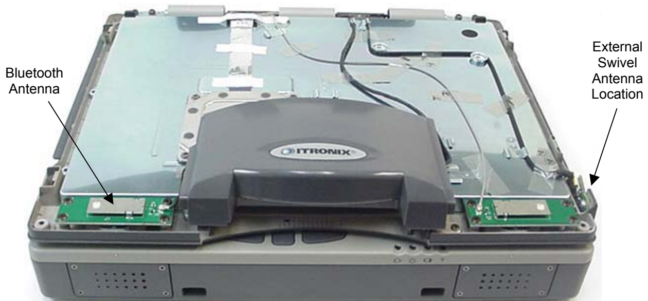
Photograph A-7 – Surface-Mount Antenna Placement
