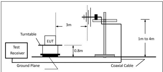
(c) For radiated emissions above 1000MHz
