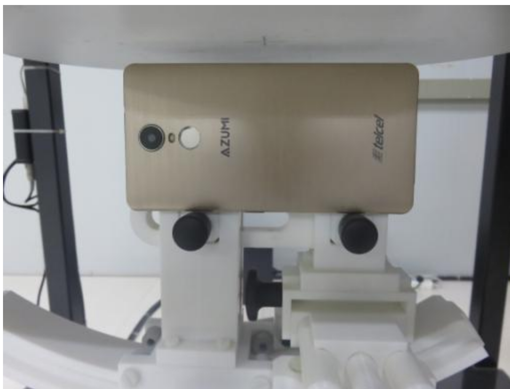
10mm body-worn Left Side Setup Photo(hotspot)
