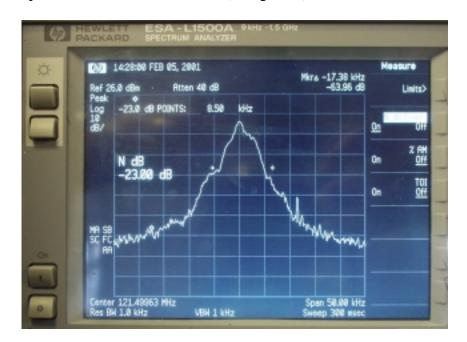
Modulation was applied with a swept signal ramping from 1KHz to 5KHz. The figure above shows that the occupied bandwidth for the 121.5MHz transmission is 8.5kHz.
