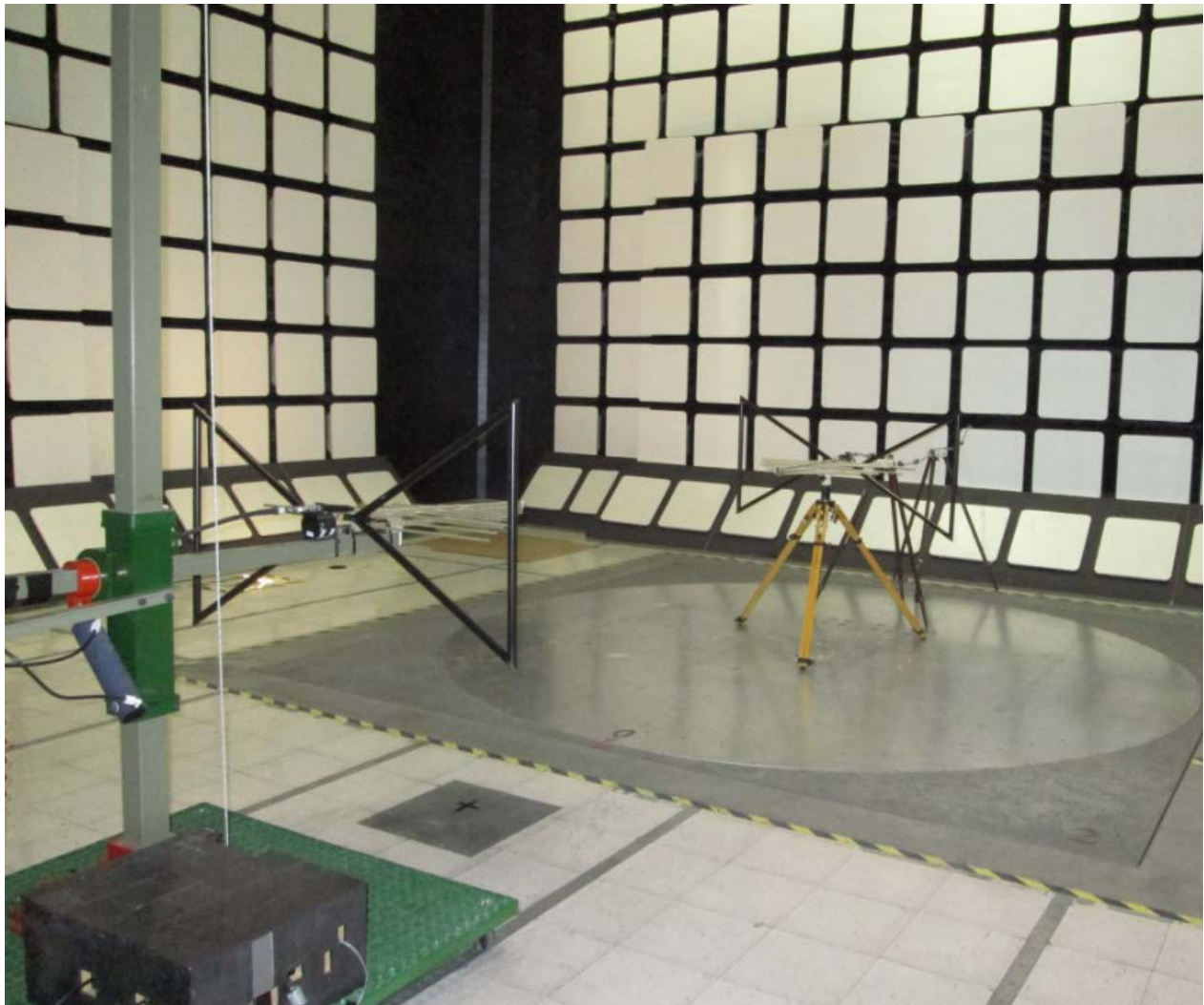
Figure 10: Substitution Measurement Setup
