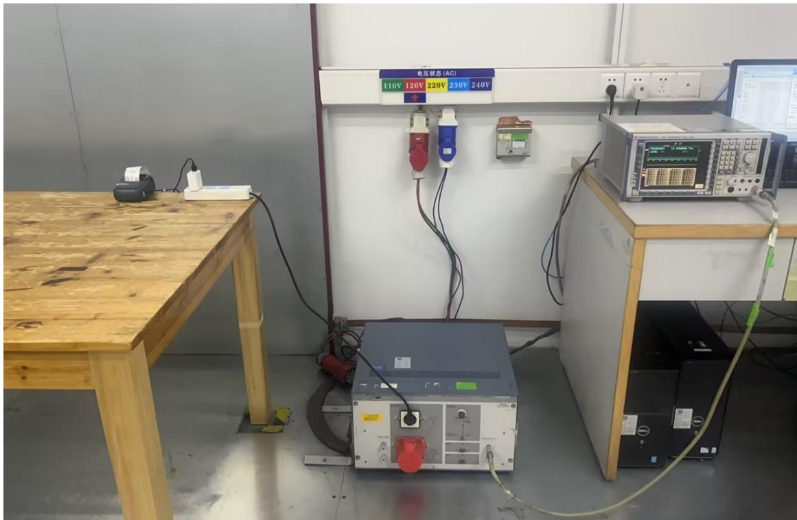
AC POWER LINE CONDUCTED TEST SETUP
