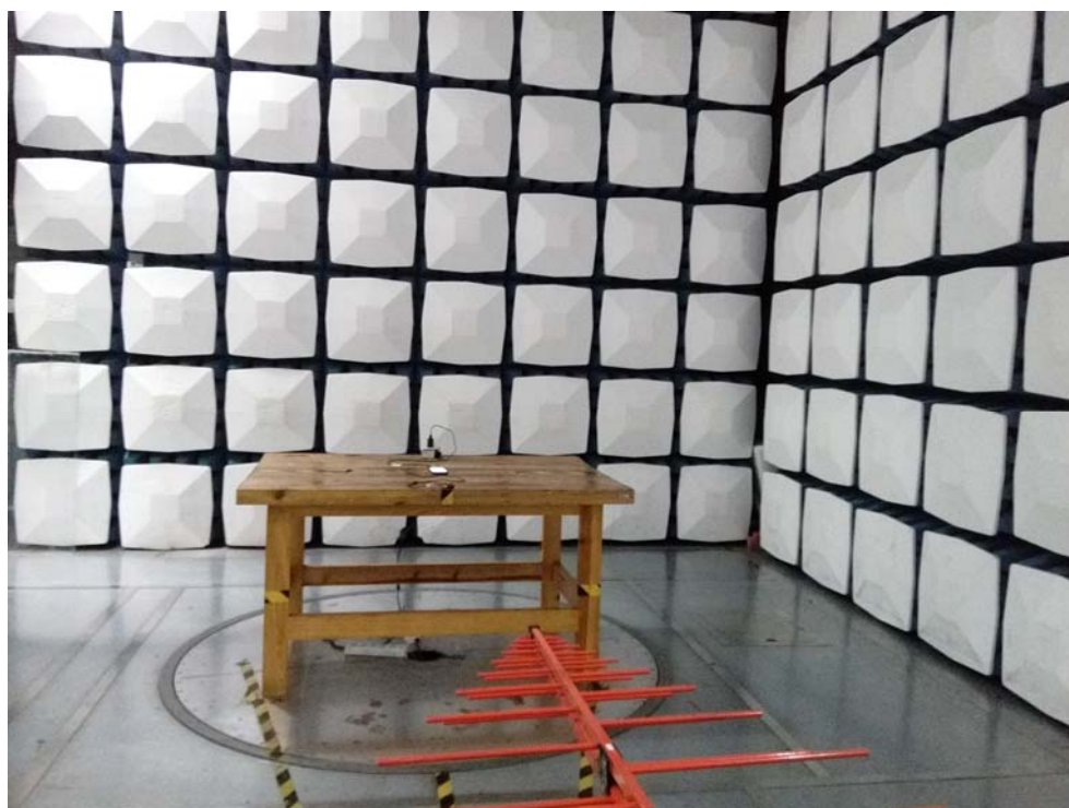
Radiated Emission Above 1GHz View
