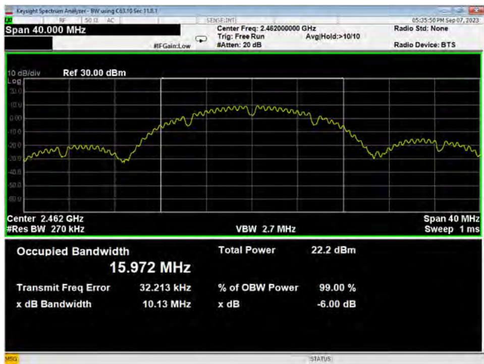
81 Occupied Bandwidth, High, Wifi B, Low Data Rate
