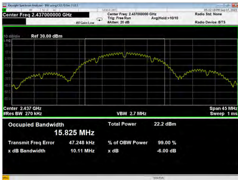
80 Occupied Bandwidth, Mid, Wifi B, Low Data Rate
