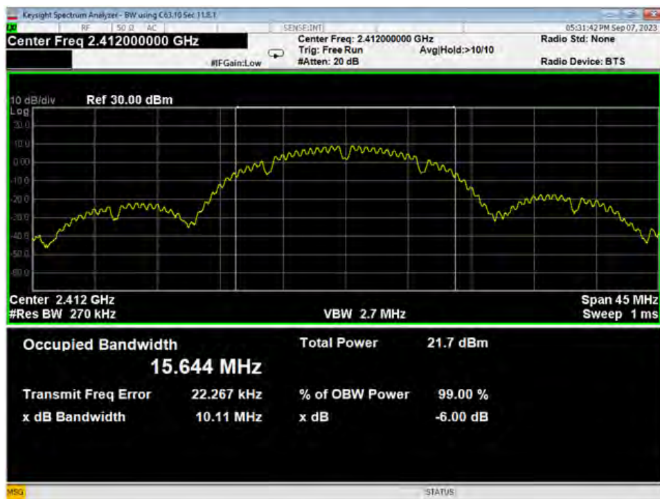
79 Occupied Bandwidth, Low, Wifi B, Low Data Rate
