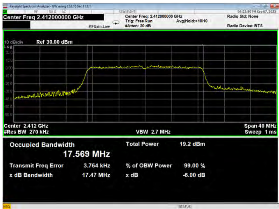
94 Occupied Bandwidth, Low, Wifi N, High Data Rate
