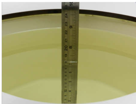
Fig 12.2 Photo of Liquid Height for Body SAR
