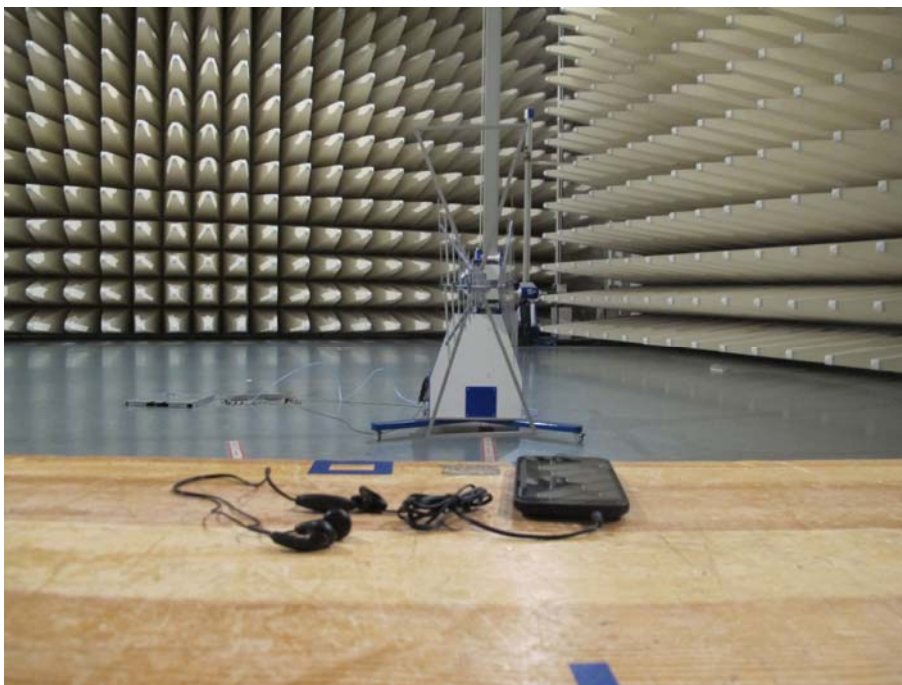
Spurious Radiated Emissions Test setup (30MHz~1GHz)
