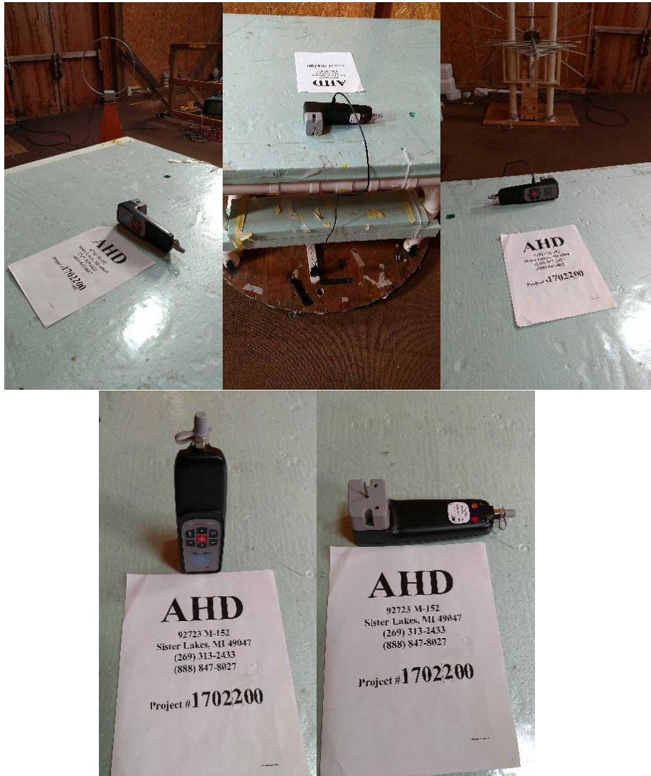
Figure 4: Radiated Emissions Test Setup Photograph(s).
