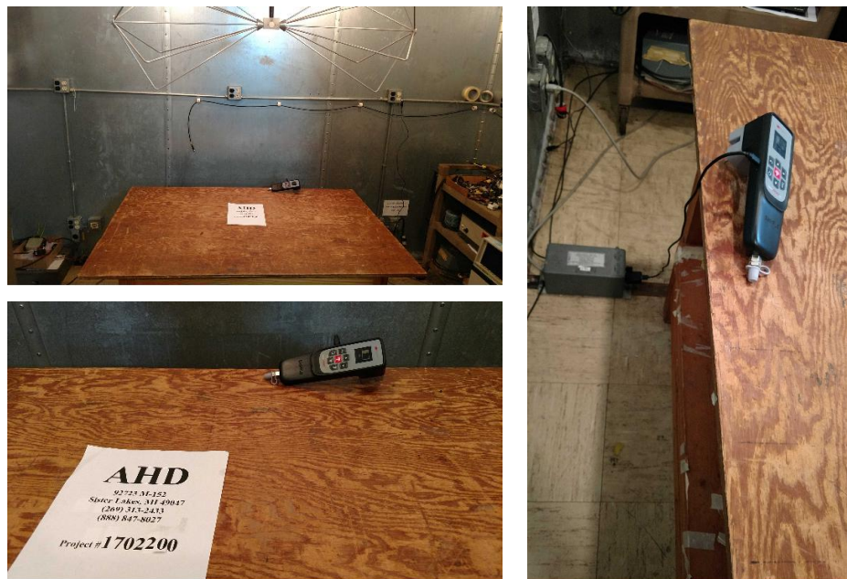
Figure 6: Conducted Emissions Test Setup Photograph(s).
